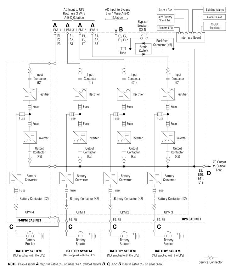
Figure 6-14. Plus 1 UPS System – Separate Rectifier Feed, Separate Battery, Dual-Feed Configuration
